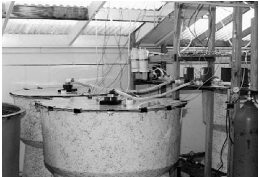
Algae was grown in covered, conical tanks made of fiberglass.
