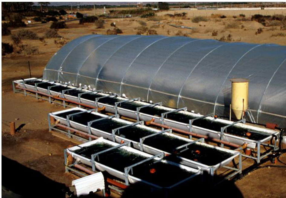
The experimental system used seaweed biofilter tanks (foreground), and an experimental fish tank under the greenhouse cover.
