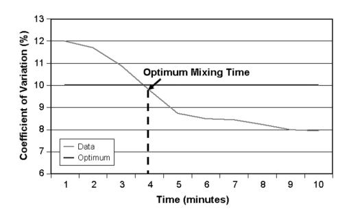
Fig. 1: This sample mixer data graph shows optimum mixing time.
