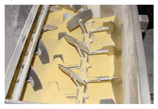
Regular examination of mixer components for wear and material build-up helps ensure clean, consistent operation. The mixing cost center is considered the heart of the feed-manufacturing process. All ground ingredients are conveyed to the center to be blended into a homogenous feed ration. It is critical that the mixing operation be performed under strict guidelines to avoid undermixing or overmixing, also known as segregation.
