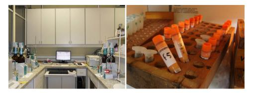
Left: View of the analytical station with titrators and central control software for pH-stat determination of protein hydrolysis at LAM-USP. Right: Ready-to-use frozen standardized enzyme extracts recovered from shrimp species for in vitro protein digestion assays at LAM-USP.
