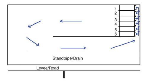
Aerial diagram of an IPRS in a traditional earthen pond. Arrows indicate water flow.
