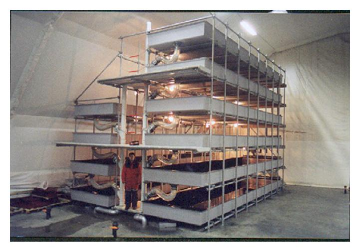
Shallow raceways can be stacked to save valuable production space. This multilevel unit is in Lofoten, Northern Norway. Photo by Dag Hansen, LOFILAB.
