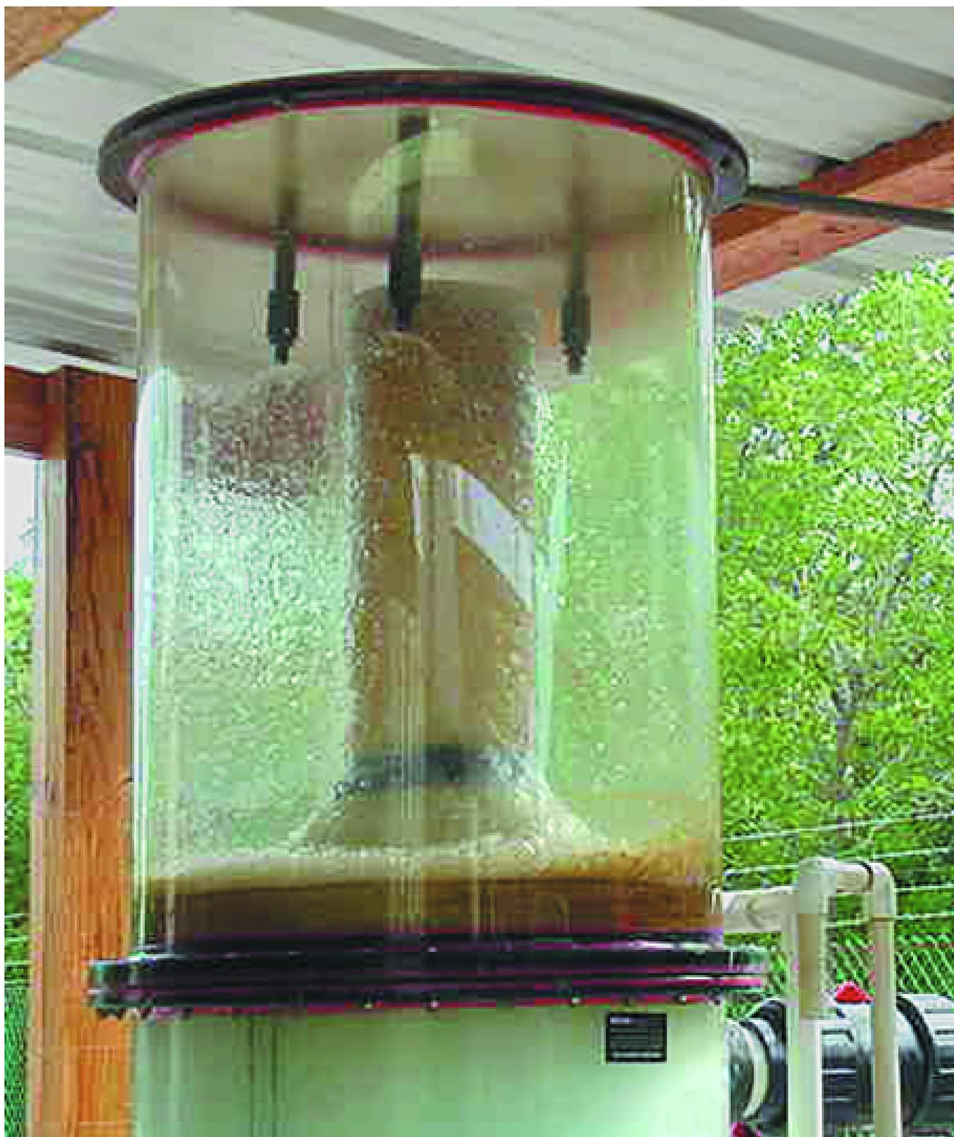
Foam action strips fine particulates in the base of this protein skimmer before the foam emerges inside the top. Spray nozzles then rinse away foam as waste.□
