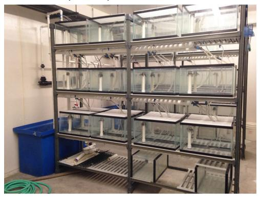
Fig. 4: One of three APL-WCAC bank systems with 37-liter aquaria and a recirculating system.
