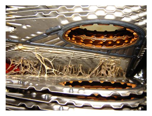
Severe biofouling of flat-plate heat exchangers can reduce efficiency to near zero.
