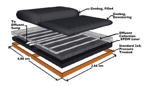
The simple construction of geotextile bag systems makes them costeffective, site-specific and mobile.
