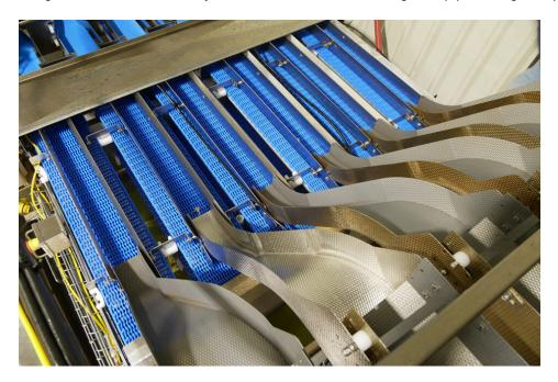
The SMART Sorter Shrimp Grader is a patented, automatically fed grader that individually images each shrimp in a lot.
