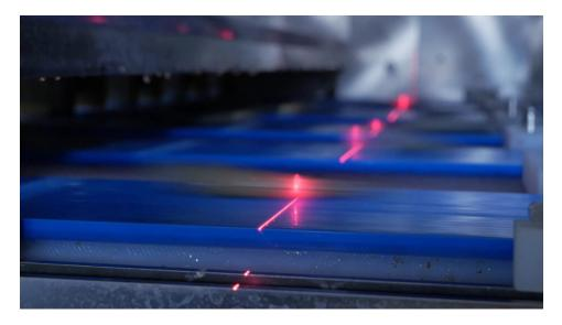
Laitram Machinery's SMART Sorter is a vision-based shrimp grader that's radically changing how shrimp processors do business. The SMART Sorter uses laser imaging and computer-vision algorithms to inspect, grade and sort shrimp in various product presentations.
