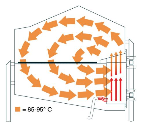
Forced convection assures reasonable cook times through the improved heat transfer provided by a steam-air mixture.
