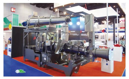
This conical rotating twin-screw extruder was designed to efficiently produce shrimp feed. An oblique tube die is attached after the back-pressure valve.
