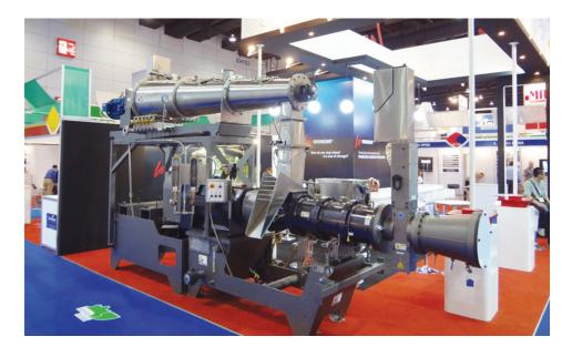
This conical rotating twin-screw extruder was designed to efficiently produce shrimp feed. An oblique tube die is attached after the backpressure valve.
