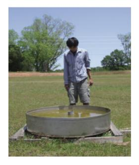
The U.S. Weather Bureau Class A evaporation pan is a common device for measuring evaporation. The amount of water lost from these pans (corrected for rainfall input) is measured daily.
