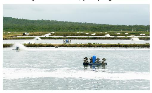
Given that aerators are often operated continuously in Australia, aeration is an important area for gaining energy efficiency.
