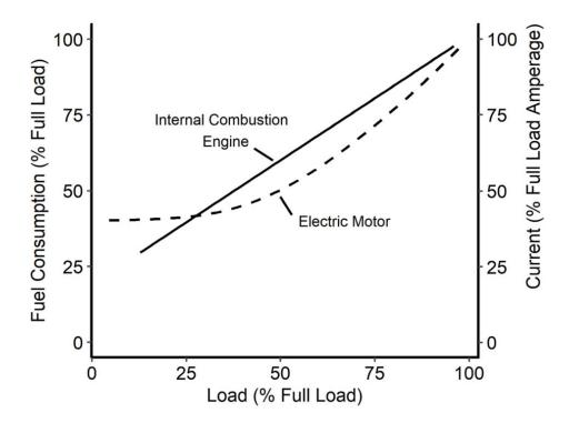
Fig. 1: Load versus fuel use by internal combustion engines and current use by electric motors (prepared with information from http://dieselserviceandsupply.com/Diesel\_Fuel\_Consumption.aspx and from
