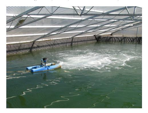
A propeller-aspirator-pump aerator.
