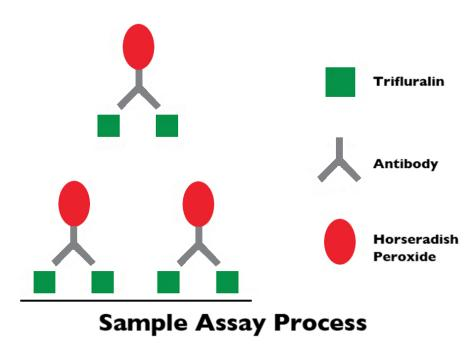
An unlabeled trifluralin conjugate is coated onto a 96-well plate. Samples are incubated in the wells, and then antigen is added. The conjugate binds to the antibody if its binding sites are not already bound by an antigen. As the amount of unlabeled antigens in the sample increases, less conjugated antigen is bound to the plate. The plate is then developed with substrate, and color change is measured.
