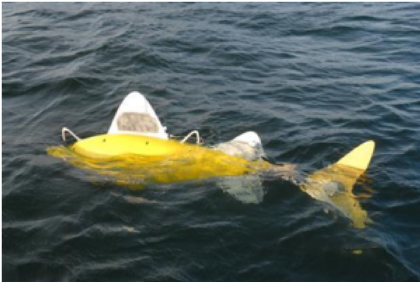
Shoal's robotic fishes work collectively using AI to locate sources of pollution underwater. Photo courtesy of SHOAL Consortium.
