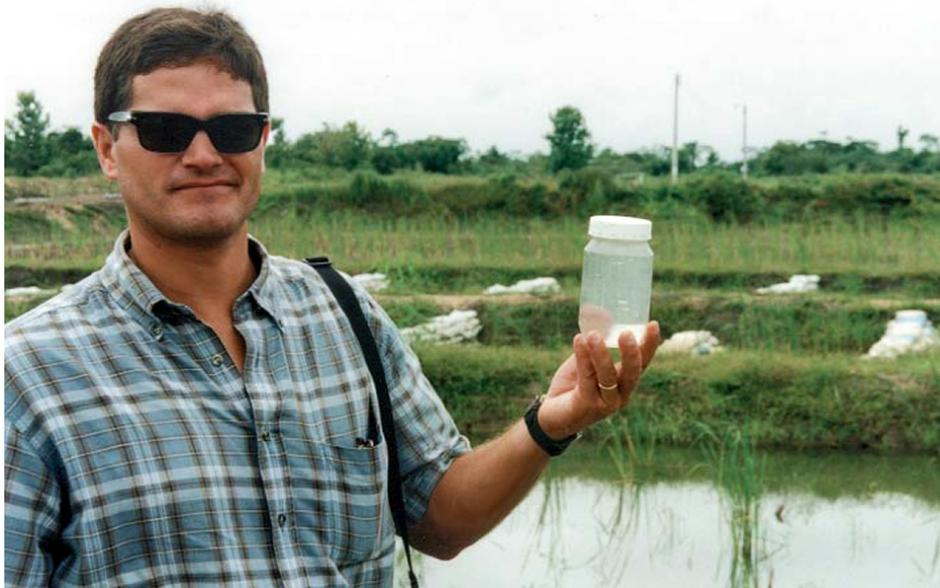
Collecting effluent water sample after passage through sedimentation area and artificial wetland (background).
