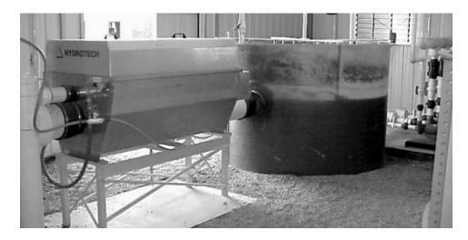
Drum filter (left) for solids removal from a recirculating system.
