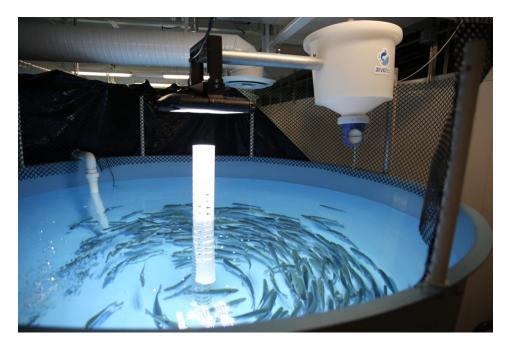
Photoperiod manipulation setup in a 5-cubic-meter tank at the University of British Columbia. Tanks are covered with a black tarp (not shown); a 168 LED lamp (20,000 lm, 5,000 K) with bright timer control is supported from the feeder stand above the center of the tank. Photo by Kevin Stiller.
