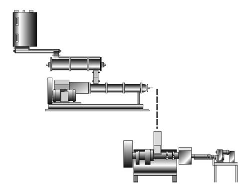
One way to produce dense, well-cooked feeds is to use separate extruders for cooking and forming.
