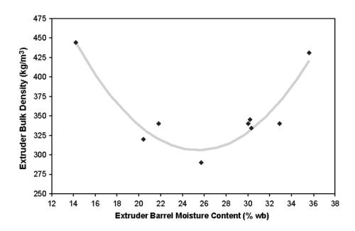
Fig. 2: Effect of extrusion moisture on bulk density.
