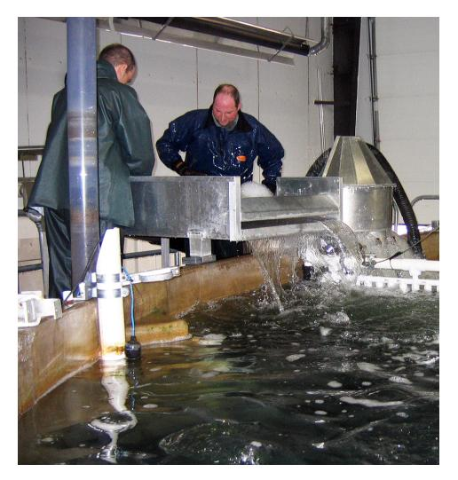
A clamshell crowder/grader constructed of PVC pipe combines with an airlift pump to quickly harvest and grade 1.35-kg rainbow trout and Arctic charr.
