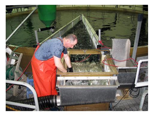
When drawn in, the V-shaped clamshell grader efficiently moves yellow perch to the side of the growout tank, where they pass to the sidewall box for harvesting.
