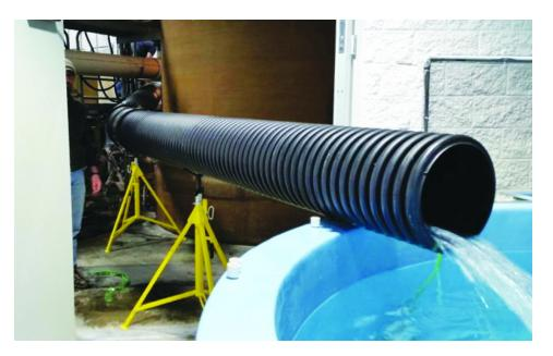
A fish transfer pipe can easily be set up to carry fish from the growout tank's sidewall harvest box to the finishing/purging tank.
