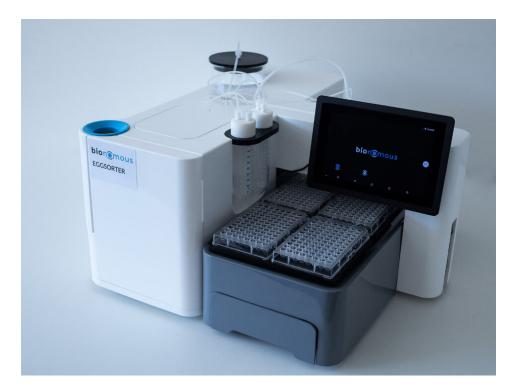
The EggSorter provides an automated solution to hatcheries for egg quality control and sorting, which are laborious tasks currently carried out manually.
