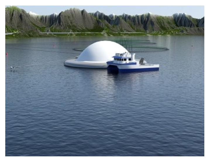
The Egg, a closed-containment system aquaculture developed by Hauge Aqua, is designed to prevent sea lice and escapes, allowing sea water to come in from the bottom.
