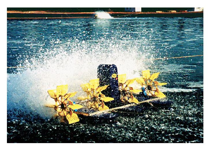
Each applied horsepower of aeration supports about 450 to 550 kilograms per hectare of shrimp production.
