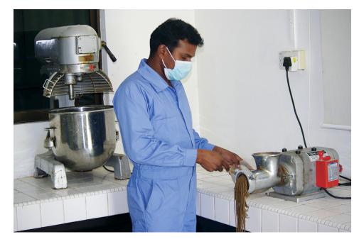
Cooked meal is fed through a meat mincer to produce feed strands. The feeds must meet internal standards for water stability and other parameters.
