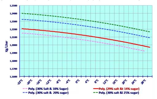
Fig. 3: Evolution of the density of four types of brine as a function of temperature.
