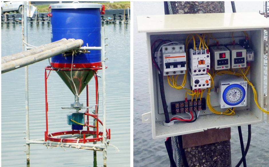
In small culture ponds, an automatic feeder can broadcast feed in a radius of 10 m and feed 600,000 shrimp. Timers control the broadcasting times and intervals of feeding.
