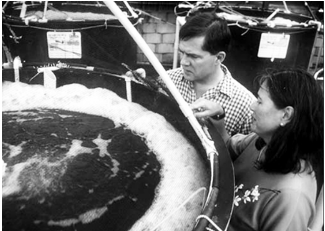
Strong aeration within CAM tanks stimulates development of a rich microbial floc.
