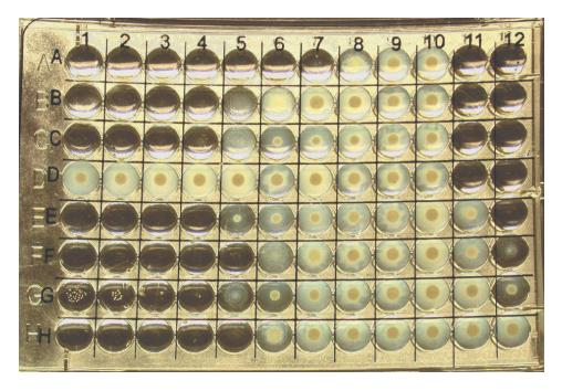
Broth microdilution tests determine minimum inhibitory concentrations in a microtiter format.
