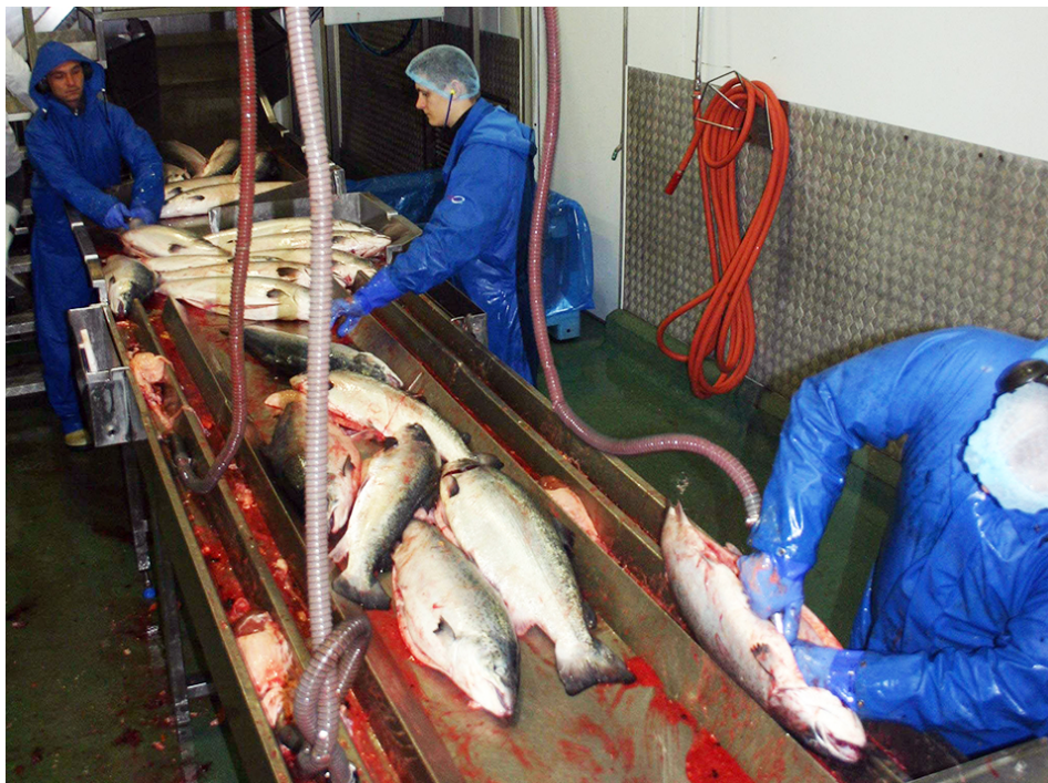
Primary processing of Atlantic salmon in Scotland removes viscera for oil extraction and hydrolysis.
