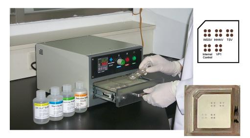
This mini hybridization oven was specially designed for multiviral biochip-based kits. The chip to right indicates the subject shrimp was infected with IHHNV and TSV.
