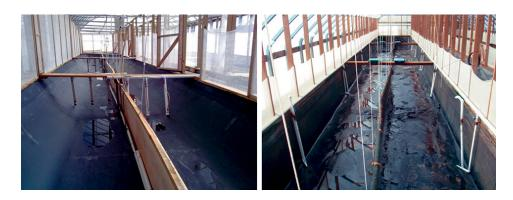
The earlier raceway system (left) used airlifts for aeration and water circulation. The newer, larger raceways utilize rows of non-Venturi injectors for water circulation.
