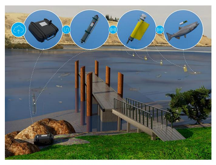
A new acoustic receiver provides timely information to dam operators and decision-makers about when, where, and how many fish are expected to pass through dams. Photo courtesy of PNNL.
