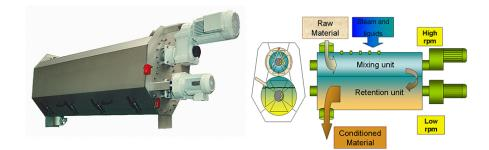
This new double-pass preconditioner for extruders features high radial mixing in a chamber where steam and water are injected. In a second chamber, more axial mixing occurs and feed meal hydrates. Photo and diagram courtesy of Buhler.
