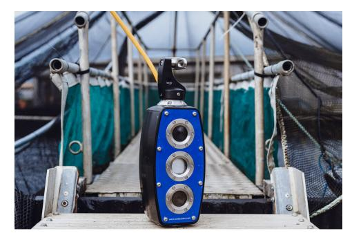
The A-BIOMASS system contains two stereoscopic cameras calibrated to take images synchronously. Through machine learning, Al identifies fish and critical points, such as tail and fins, to measure fish height, weight and length accurately.
